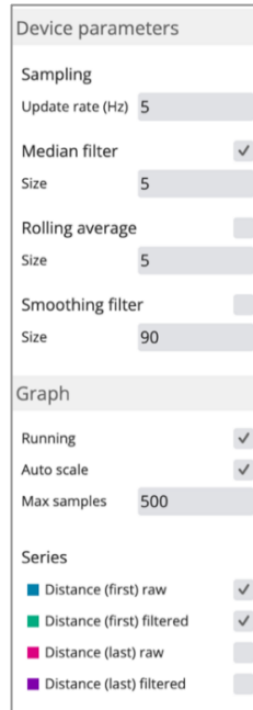
Figure 12: LightWare Studio GRF-250 parameters page
