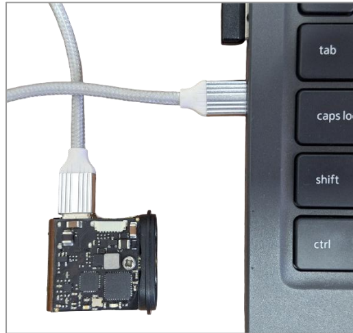
Figure 8: GRF-250 connection to the USB port
