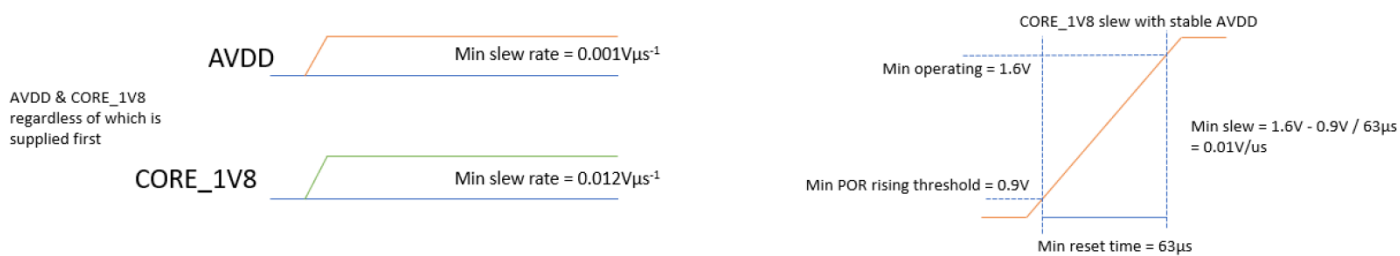
Figure 9. Power up slew
