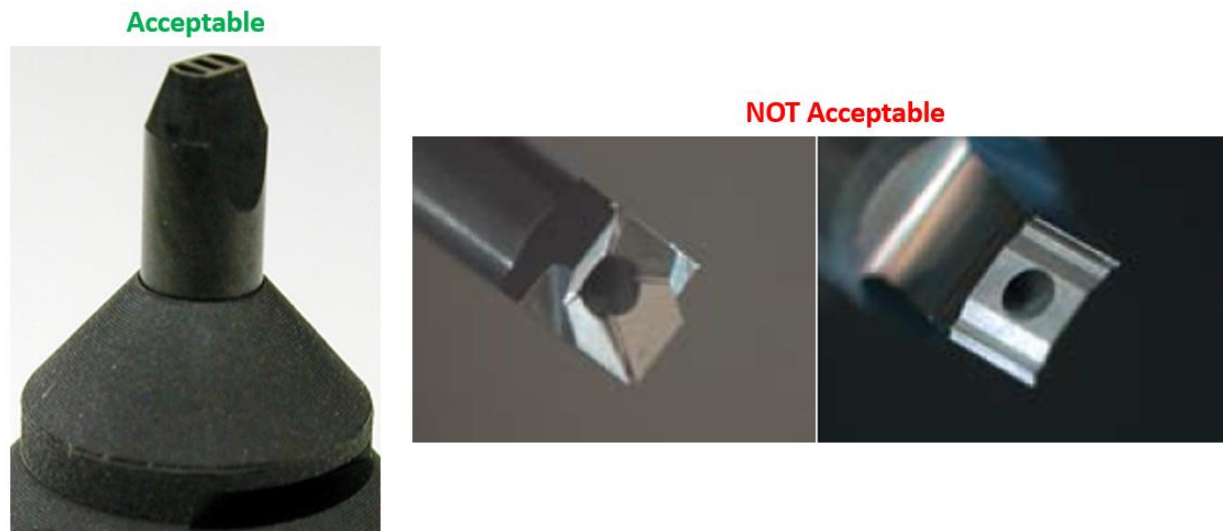
Figure 7: Acceptable vs. NOT Acceptable Tip Shapes
